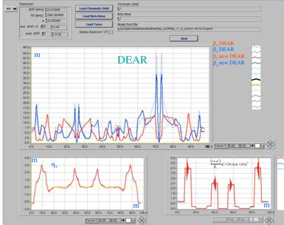
Figure 1: DEAR optics evolution presented by the Control System model interface.
