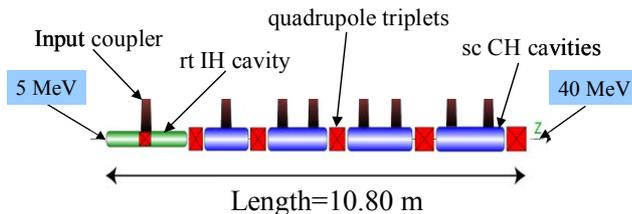
Fig. 2: Scheme of a 175 MHz sc IH/CH-DTL.
