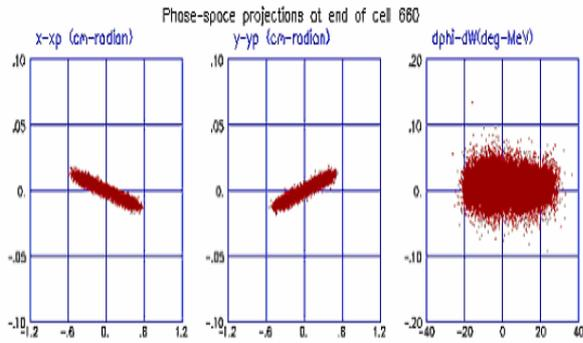
Fig. 1: Output distribution at 5.0 MeV of the Four-Vane-RFQ, calculated with 50000 macro particles.
