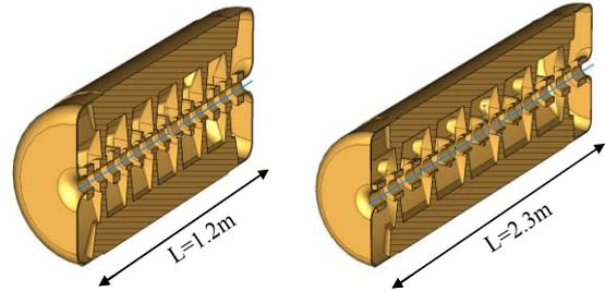
Fig. 3: 3D view of the first and last 175 MHz sc CH-cavities (tank 1 and 4) calculated with Microwave Studio®.
