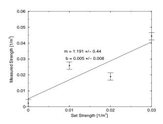
Figure 2: Sextupole calibration curve obtained with difference orbits collected during the RHIC 2003 dAu run.
