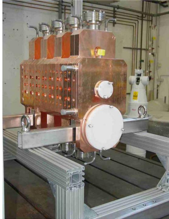
Figure 2: Segment at final dimension control
