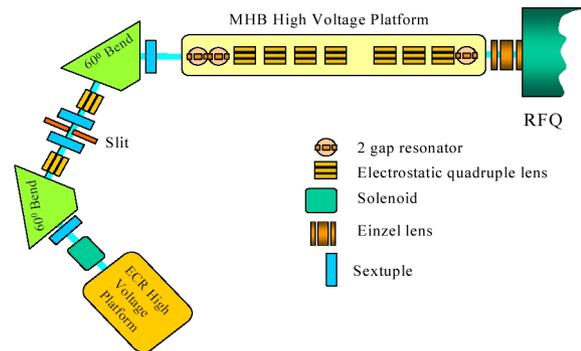
Figure1: Schematic layout of RIA driver LEBT
