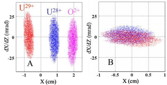
Figure 3: Transverse phase space plots in bending section. (A) at slit position shown in Fig.1. (B) – at MHB entrance.
