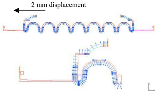
Figure 2: Loads on cold cavity
