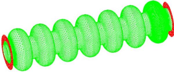
Figure 5: Shell mesh on high gradient cavity
