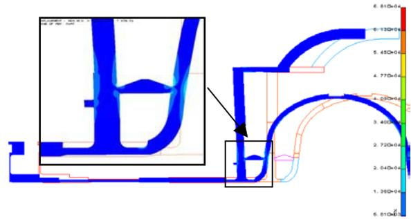
Figure 3: Low Loss – 2 mm deflection + 4 atm load
