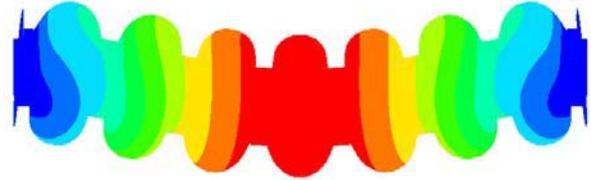
Figure 6: Fundamental mode of high gradient cavity
