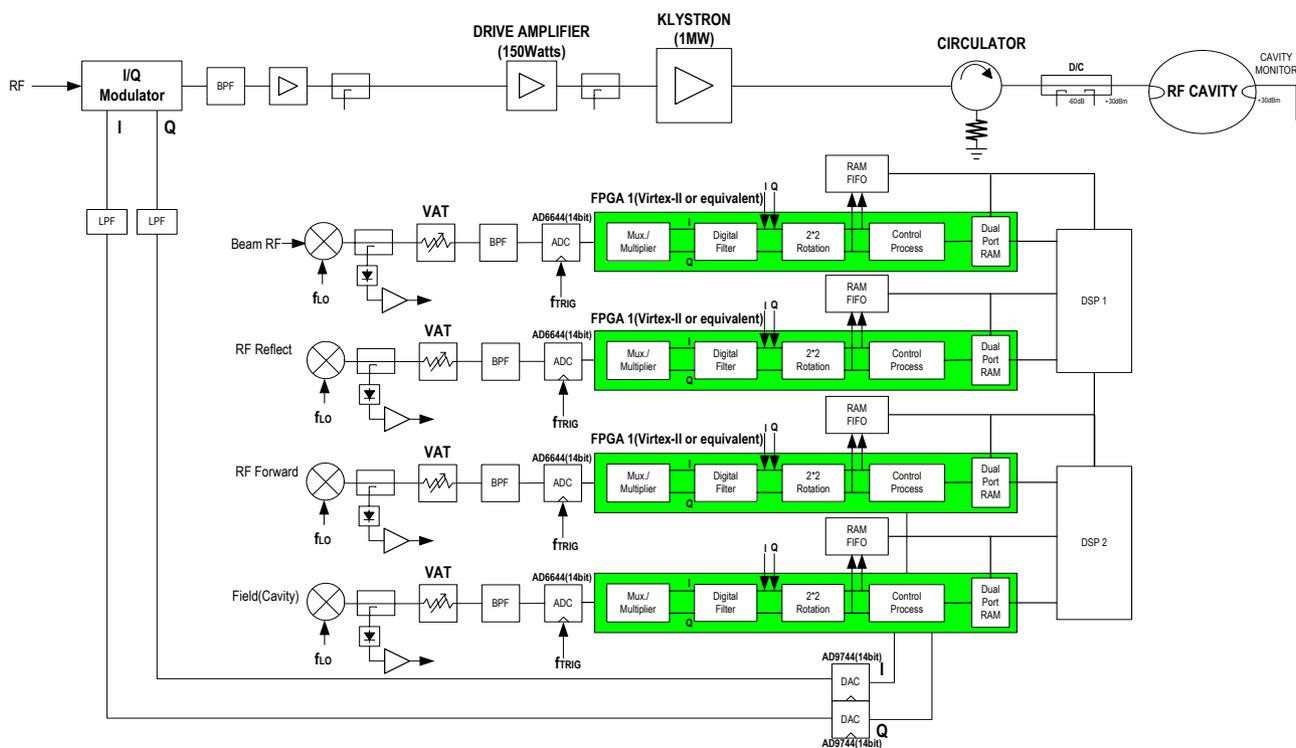
Fig. 2. A block diagram of the digital feedback hardware
