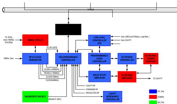
Fig. 3. The interface of the RF station for the RFQ, DTL1, DTL2.
