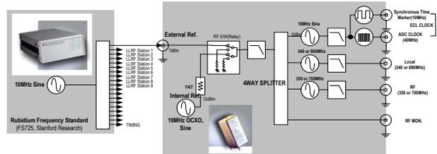
Fig. 1. A block diagram of the master oscillator and RF generator included 40MHz ECL clock for 100MeV linear accelerator
