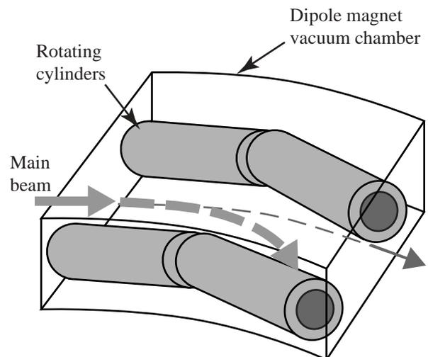
Figure 2: Beam dumps located in the first dipole magnet cavity.
