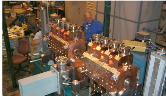
Figure 8. Bead Pull measurement on the Hot Model
