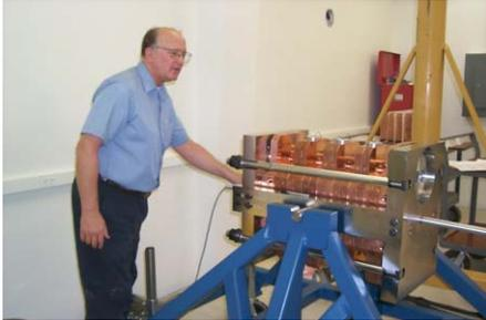
Figure 5. Measuring the Segment Frequency
