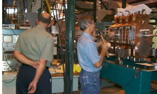
Figure 7. Tuning the Accelerating Cells
