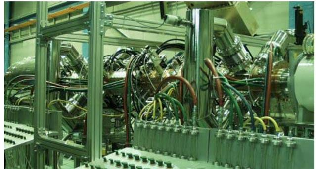
Figure 3. Assembled 3.0MeV RFQ system.
