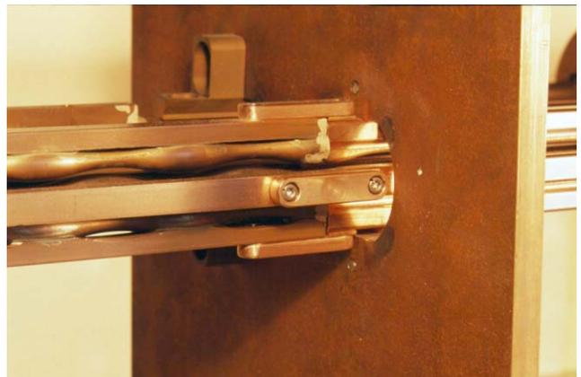
Fig. 8: The mounted electrodes at the stem.
