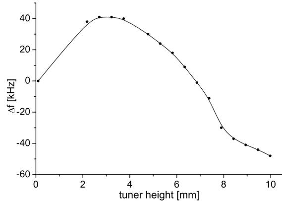
Figure 6: Frequency tuning of the CH cavity by a cylinder as shown in Fig.5 with variable height
