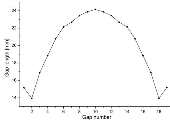
Figure 3: Gap length distribution along the CH cavity at a constant periodical length of 42.857 mm
