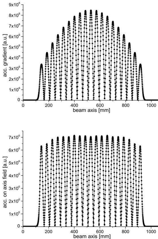
Figure 2: Accelerating on axis field distribution of the 352 MHz CH cavity without (top) and with (bottom) gap length variation
