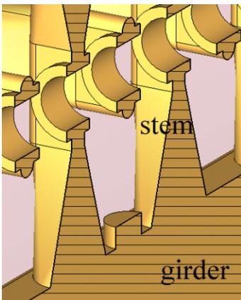
Figure 5: Tuning the 352 MHz CH cavity with cylindrical niobium blocks along the girders
