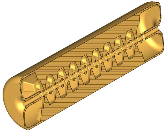
Figure 1: The sc 352 MHz CH prototype with matched end cell geometry
