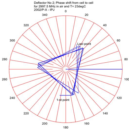
Fig.5 The measured phase advance per cell in second deflecting structure of CTF3
