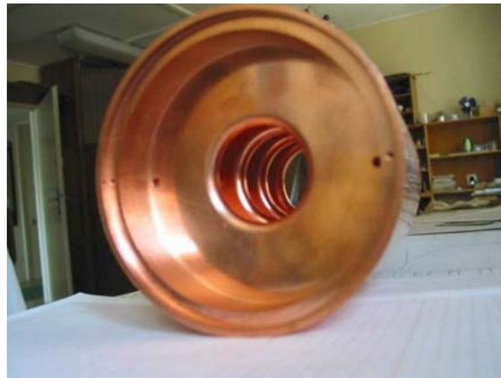
Fig. 2 The pilot series of 4 cells after hydrogen furnace brazing with  $880^{\circ}\text{C}$  LV30P filler alloy.
