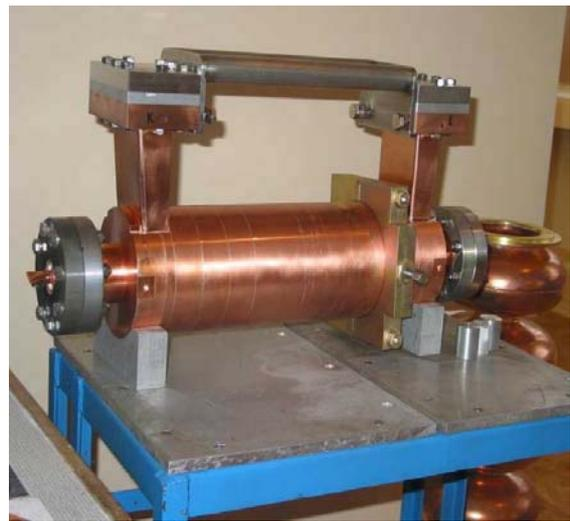
Fig. 4 3 GHz deflecting structure after fabrication
