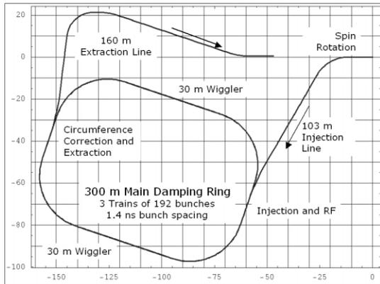
Figure 1: Overall Layout of the Electron MDR
