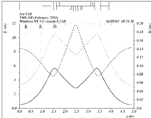
Figure 2: Lattice Functions in One Arc Cell
