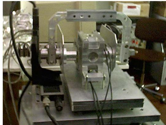
Figure 2: BPM calibration bench
