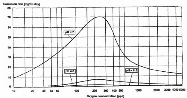
Fig. 2: Influence of dissolved oxygen on copper release rate. [20]
