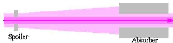
Figure 6: Spoiler type collimator [27].
