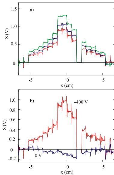
Figure 3. PAPS profiles with a) three background pressures increasing in ascending order from 0.4  $\mu$ Torr to 1.2  $\mu$ Torr 1 ms after injection, and b) -400 V and 0 V on the H.V. plate, 2 ms after injection. Ch. 11 is inactive.
