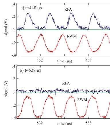
Figure 4: RFA and RWM data recorded just after injection,  $V_{ret} = 0$  V,  $V_{col} = 30$  V (1 M $\Omega$ ), a)  $t_{start} = 448$   $\mu$ s, b)  $t_{start} = 528$   $\mu$ s. The signals are temporally aligned.
