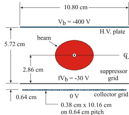
Fig. 2. Horizontal Profile and Position System (PAPS).
