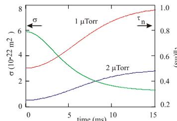
Figure 1: Ionization cross section and neutralization times in the RCS for 1 and 2  $\mu$ Torr, N<sub>2</sub>.
