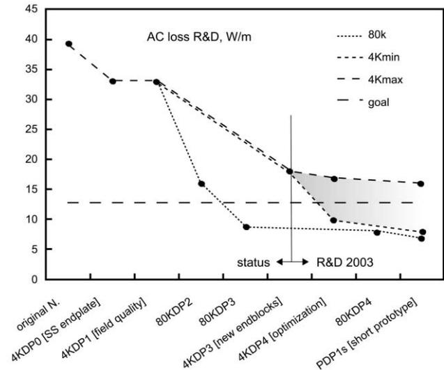
Figure 1 : A significant reduction of the dynamic losses of the Nuclotron magnet has been achieved.
