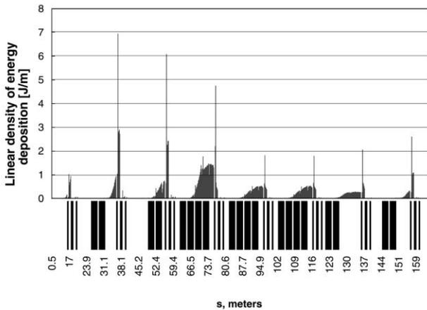
Figure 3 : Calculated distribution of beam loss induced energy deposition in one arc of SIS100, assuming 5% losses of the initially  $10^{12} U^{28+}$ -ions.
