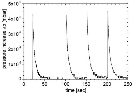
Figure 2 : Measured beam desorption induced total pressure increase in the test-stand. Shown is the pressure rise by the irradiation of a Cu sample with a 1.4 MeV/u  $C^{2+}$ -beam.
