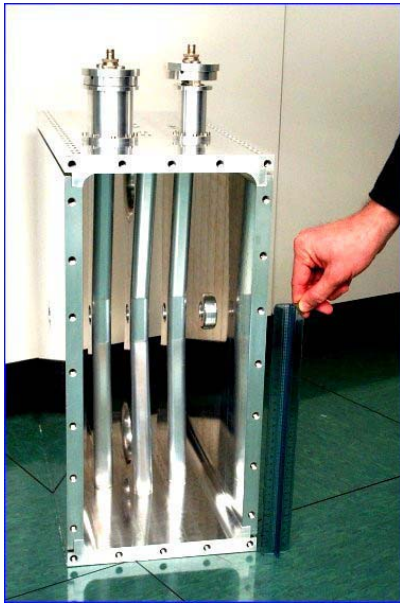
Figure 6: A 352 MHz, four-gap 'ladder resonator' for \beta=0.12 is being developed at INFN-Legnaro
