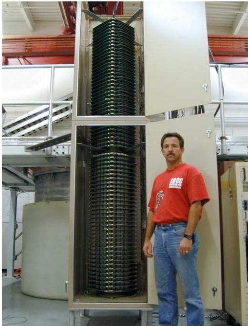
Fig. 2: Single-stack 50 kV modulator
