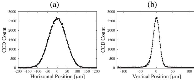
Figure 4: (a) horizontal and (b) vertical beam profiles with their fitted gaussian curves. Data from 2002/06/06.
