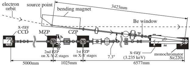
Figure 2: Layout of the beam profile monitor system.
