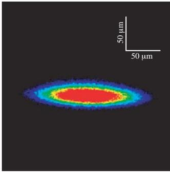
Figure 3: Electron beam image obtained by the beam profile monitor. The length of the horizontal and vertical white bars corresponds to 50  $\mu\text{m}$  at the SR source point.
