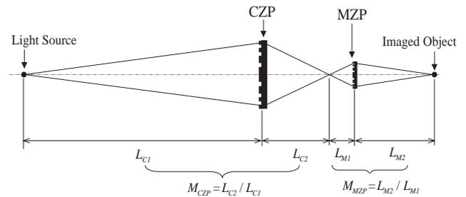
Figure 1: Imaging optics of the beam profile monitor.
