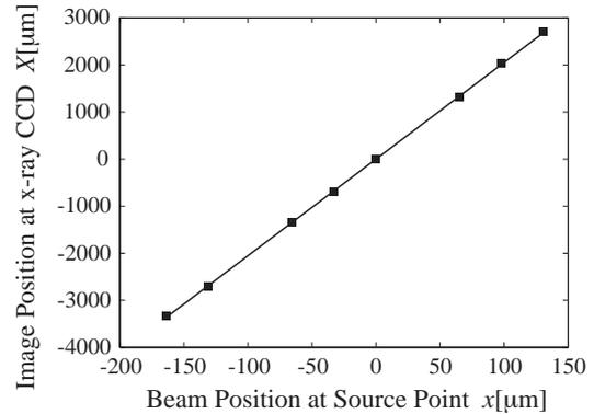
Figure 5: Relation between the horizontal beam position at the SR source point and the horizontal position of the beam image on the x-ray CCD. Data from 2002/05/30 - 06/07.
