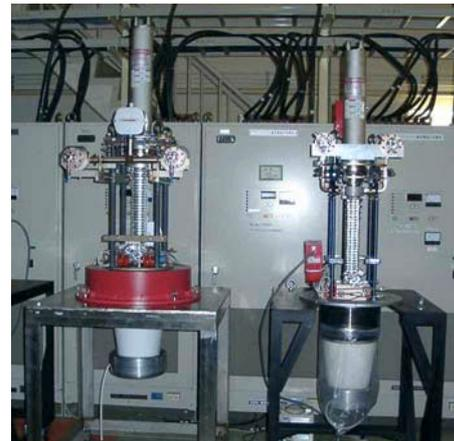
Figure 4: Photo of the first (PPM-1, right) and the second (PPM-2, left) PPM klystrons for GLC.
