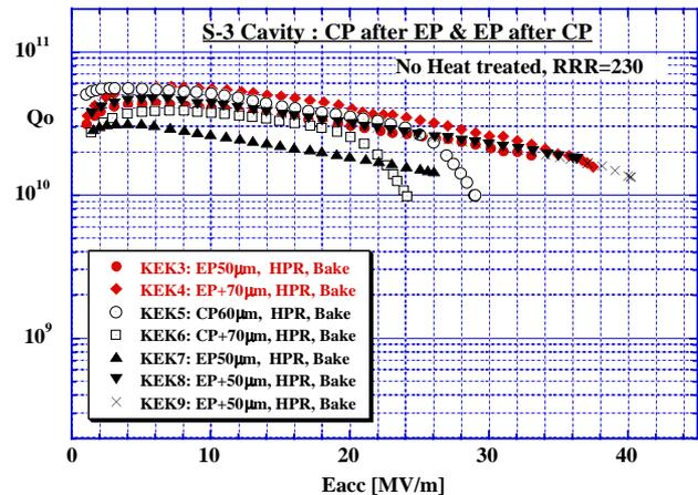
Figure 7: Evidence of the superiority of EP over CP with high gradient performance.
