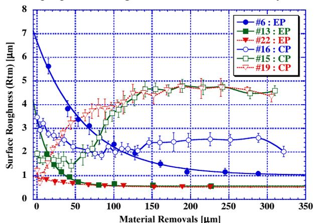
Figure 1: Surface roughness of niobium by EP or CP.
