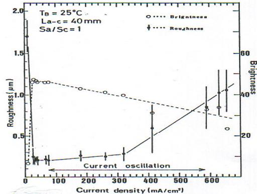
Figure 4: Optimum current density of niobium EP.
