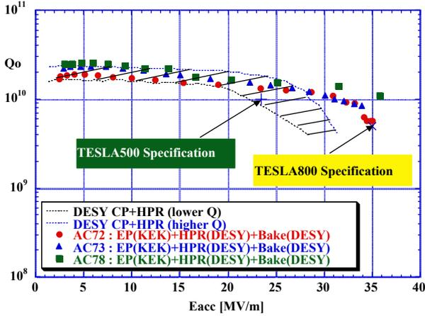
Figure 8: Results of electropolished TTF cavities.
