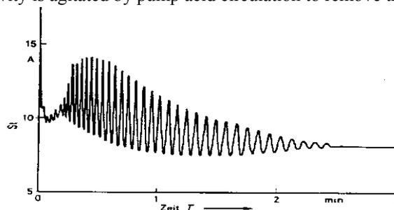
Figure 3: Current oscillation appeared in EP of niobium.
