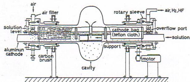
Figure 5: Horizontal rotated continuous electro-polishing.
