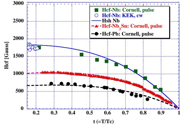
Figure 10: Critical RF fields ( $H_{cf}$ ) of sc cavities and  $H_{sh}$ .
