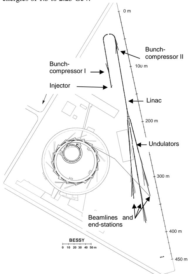
Fig. 1: Overview on the FEL adjacent to the present 3<sup>rd</sup> generation SR-source BESSY II operational since 1998.
