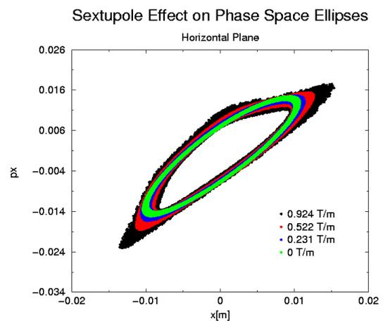
Figure 2: Horizontal phase space ellipses at one location of the ring after tracking for 62530 turns with different sextupole strengths. The nominal sextupole strength of 0.522 T/m is represented by the red ellipse
