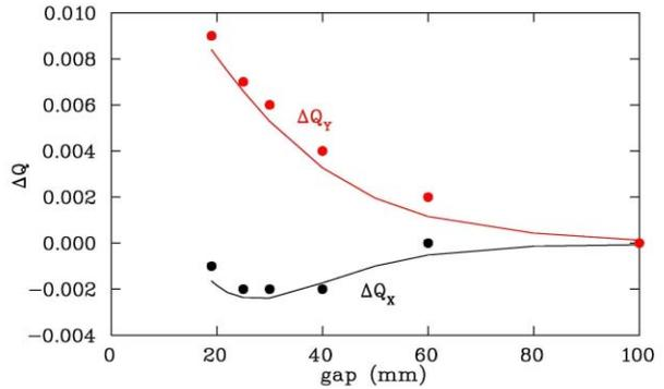
Figure 5: Measured (dots) and computed (lines) tune shifts as a function of the gap for one undulator segment at 2 GeV (black=horizontal plane, red=vertical).
