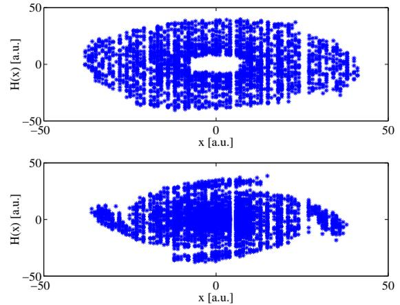
Figure 8: Comparison of the horizontal phase spaces with the undulator open (top) and closed (bottom) with  $Q_x = 14.25$ .
