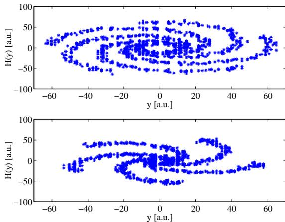
Figure 6: Comparison of the vertical phase spaces with the undulator open (top) and closed (bottom) with  $Q_y = 8.20$ .
