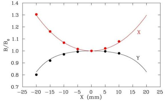
Figure 4: Measured (dots) and computed (solid line) transverse field distributions at minimum gap.
