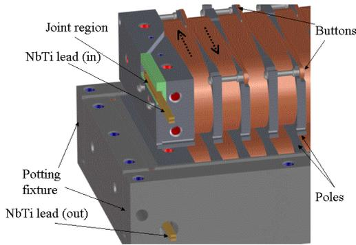
Figure 4 Model of the LBL 6-period Nb<sub>3</sub>Sn prototype.
