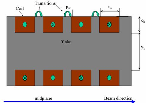
Figure 1 Superconducting undulator upper-halfplane.
