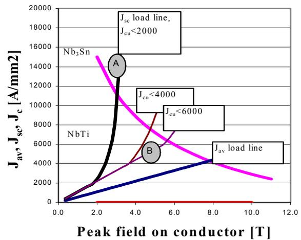
Figure 3 Effect of a copper current density limitation on the attainable performance of a device. The model corresponds to a linear B(J) load line and assumes Cu:SC=1 at low current. Once the  $J_{cu}$  limit is attained, the copper cross section is “increased “ to keep  $J_{cu}$  constant.
