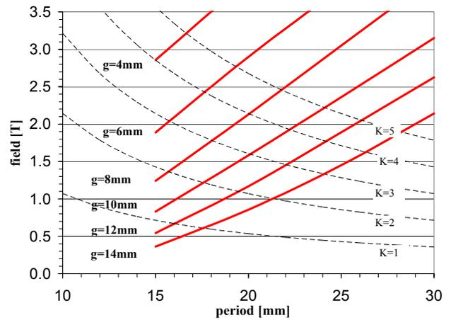
Figure 2. Performance curves for Nb<sub>3</sub>Sn superconducting undulators (see text for assumptions)
