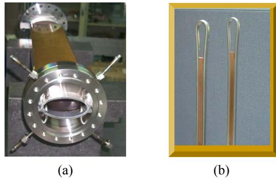
Figure 2: Photos of (a) the kicker chamber with the absorber, and (b) the cold head of the absorber.
