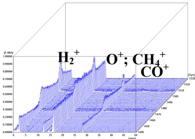
Fig. 6: RGA spectrum in mass range of 1 ~ 50 amu/e. The dominant residual gases include H<sub>2</sub>, CO, and CH<sub>4</sub>.
