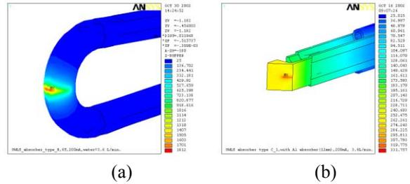
Figure 4: Thermal analysis by ANSYS for the absorber (a) without Cu cover, and (b) with both Cu cover and upstream absorber.
