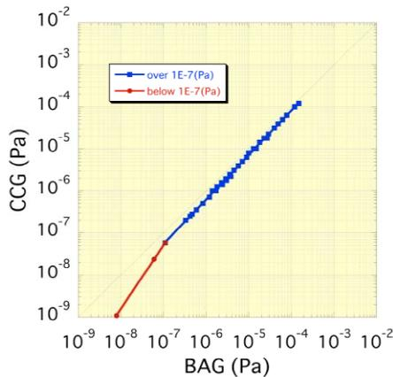
Figure 2a: CCG Calibration with Prototype Controller
