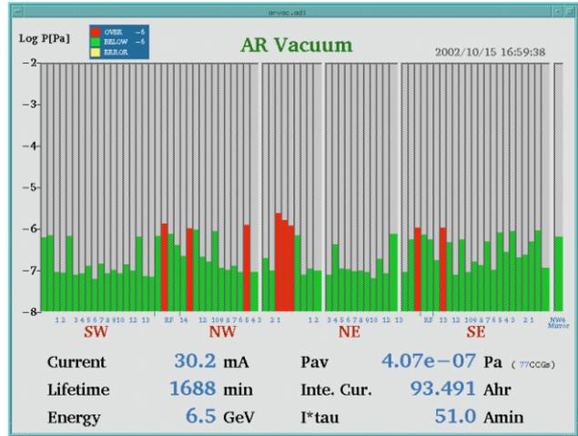
Figure 3: Ring Pressure Monitor Panel
