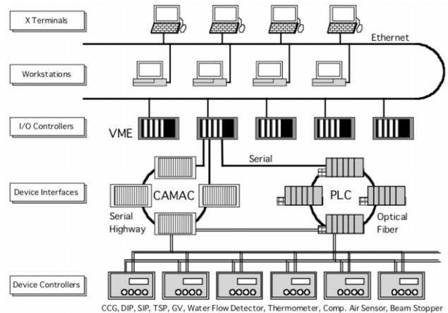
Figure 4: Diagram of Vacuum Control System
