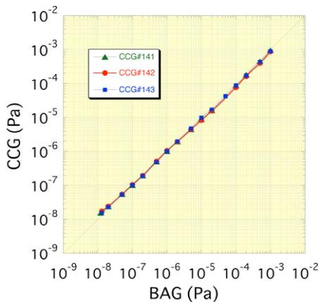
Figure 2b: CCG Calibration with Final Version Controller
