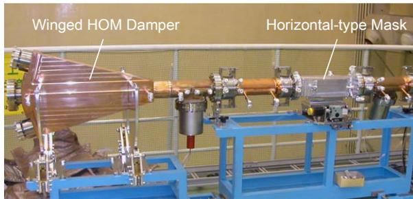
Figure 2: Winged HOM damper combined with horizontal-type movable mask.
