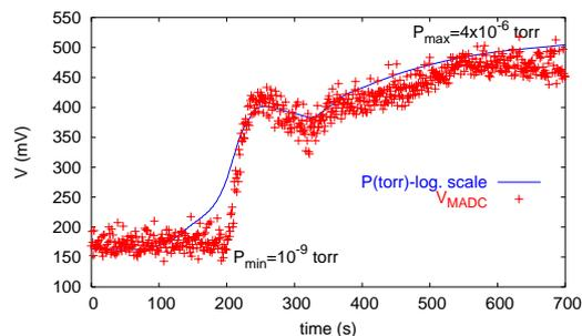
Figure 4: *EC* signal using MADC in bo2 sector while filling RHIC with 110 bunches. Injection was temporally interrupted after 45 bunches ( $t=200s$ ) and resumed at  $t=320s$ . Note that  $P$  is plotted in logarithmic scale.
