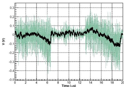
Figure 3: *EC* signal on the *ED* placed in the bo2 sector. The light dotted green line shows the raw data, whereas the black solid line shows the smoothed data using a numerical 10 MHz filter.
