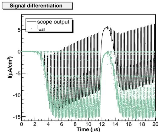
Figure 2: Theoretical  $I_{wall}$  calculated with *CSEC* (green light dots). This signal is differentiated by the RHIC ED system, and has been evaluated with *PSPICE* (black line).
