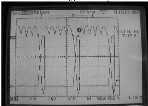
Figure 8 Capacitor current  $i_{cs}$  (240A/div) and output current  $i_o$  (140A/div)
