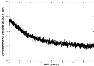
Figure 2 : Long-term stability of output current after adding extra control loop
