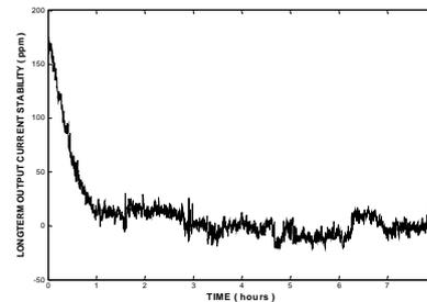
Figure 3 : Long-term output current stability after modification of reference input stage
