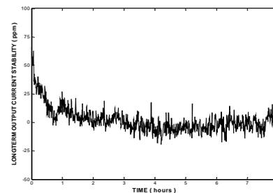
Figure 4 : Long-term output current stability after replacement of DCCT
