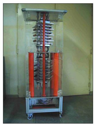
Figure 1: LTT crowbar assembly consisting of two stacks mounted vertically.
