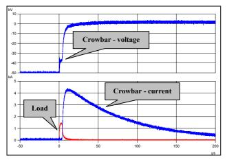
Figure 5: Crowbar operation at nominal voltage
