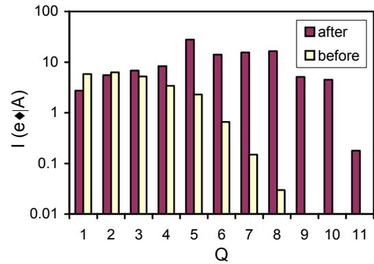
Fig. 5. Comparison of charge-state distributions for  $Ar$  ion beams extracted from the conventional minimum- $B$  configuration before and after improvements made to the source.
