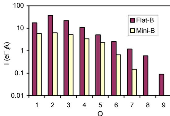
Fig. 4. A comparison of  $Ar$  charge states obtained with flat- $B$  and conventional minimum- $B$  ECR configurations.
