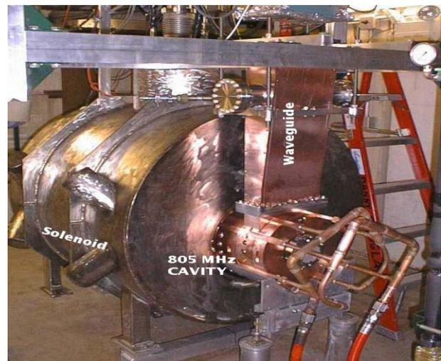
Figure 2: Solenoid and 805 MHz RF cavity
