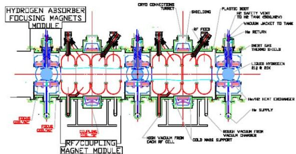
Figure 3: Mucool/MICE SFOFO lattice cell
