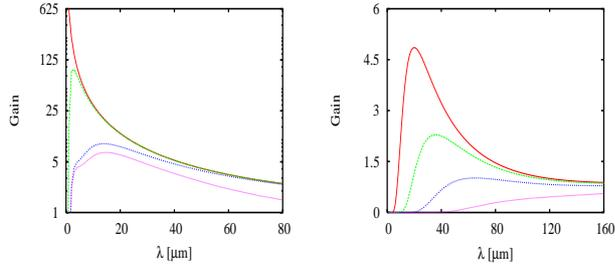
Figure 1: Gain of a model chicane as a function of the modulation wavelength  $\lambda$ . Here all used parameters are summarized in Table 1 where four numbers in a column are the parameters of red, green, blue, and magenta lines, respectively. More details can be found in Ref. [7].
