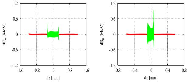
Figure 3: ELEGANT results with  $2 \times 10^6$  macroparticles: change of the uncorrelated energy deviation  $dE_u$  in the SCSS BC Phase-I (left) and Phase-II (right). Here red and green dots are  $dE_u$  before and after the BC, respectively.
