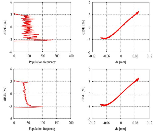
Figure 2: ELEGANT results of SCSS BC at the Phase-II stage with  $5 \times 10^4$  macroparticles (upper row) and  $2 \times 10^6$  macroparticles (lower row): (left column) population frequency versus the relative energy deviation after the BC (right column) longitudinal phase space after the BC. Here all initial conditions except the macroparticle number are the same for two cases. The main parameters are summarized in Table 2, and others are summarized in Ref. [1].
