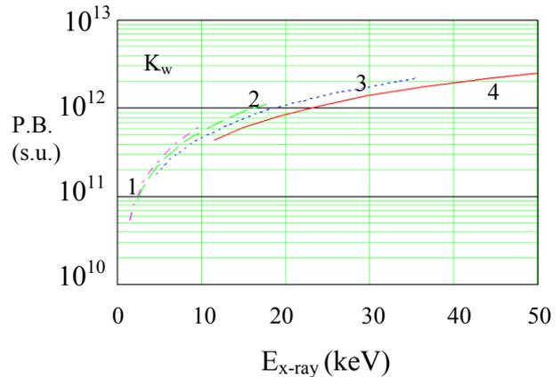
Figure 2: Peak brightness curves for Thomson x-rays generated in the wiggler of the Upgrade FEL, in standard units (s.u.): x-rays/sec/mm<sup>2</sup>/mrad<sup>2</sup>/(0.1% bandwidth). Input to these calculations include electron beam energy from 75 MeV to 125 MeV, intra-cavity IR power of 65 kW, and bunch frequency of 75 MHz.
