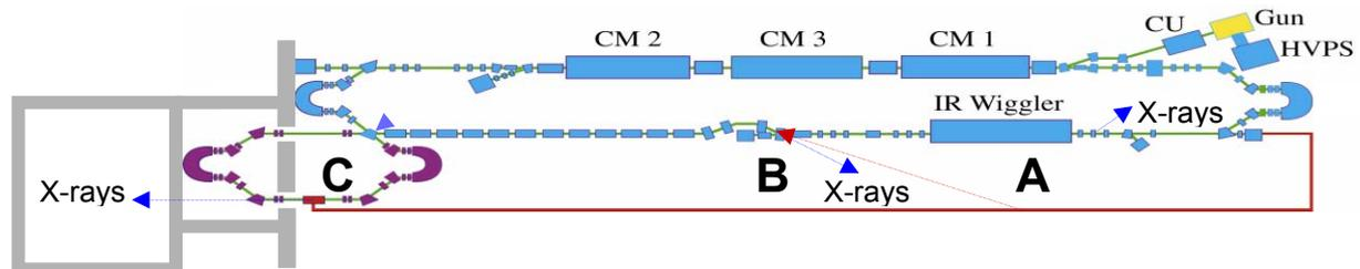
Figure 1: The Jefferson Lab Upgrade FEL layout (modified) with three site locations for Thomson x-ray sources. A) is intra-cavity production by the IR in the cavity automatically focused onto the electron beam. B) requires extracted IR brought to focus onto the electron beam in the chicane. C) has extracted IR brought to the loop and allows both beams to be focused to the smallest rms size.
