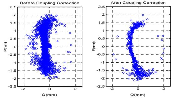
Figure 3: Poincaré surface of the section in the resonant processing frame derived from  $(x, x')$  and  $(y, y')$ , where  $Q = \sqrt{2J_1\beta_x} \cos \phi_1$ ,  $P = \sqrt{2J_1\beta_x} \sin \phi_1$ . The overall coupling phase is  $15^\circ$  and  $90^\circ$  to have the upright cross section before and after correction, respectively.
