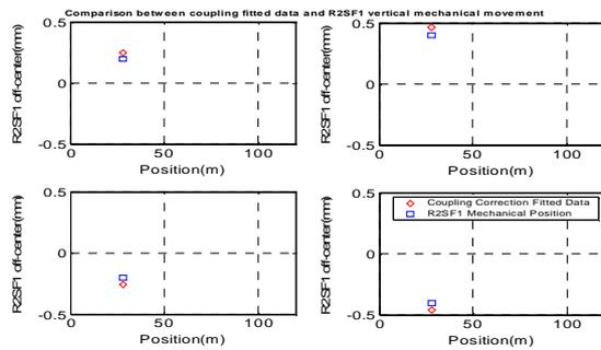
Figure 6: A comparison between the girder movement in one sextupole and coupling fitted data.
