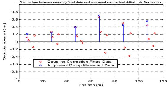
Figure 5: Girder movement data and fitted sextupole vertical position changes. The survey data is with resolution of 0.05 mm.
