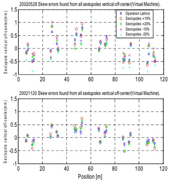
Figure 4: Fitted sextupole vertical position changes at different sextupole setting. Data taken on different date are compared.
