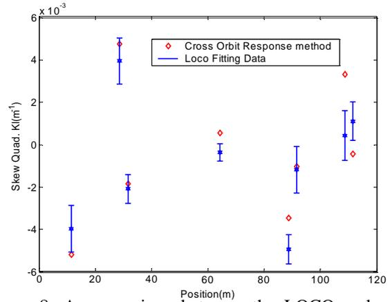
Figure 8: A comparison between the LOCO and cross orbit response analyses results for the correction skew quad strengths.
