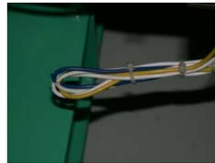
Figure 4: Cracked cover of interlock wire.
