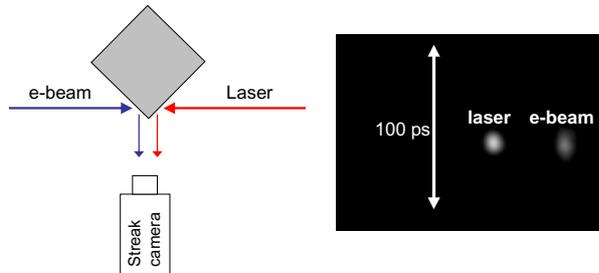
Figure 3: E-beam to laser synchronization measurement.
