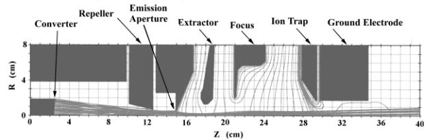
Fig. 1. PBGUNS trajectory simulations for the prototype axial H<sup>-</sup> source used in these measurements.
