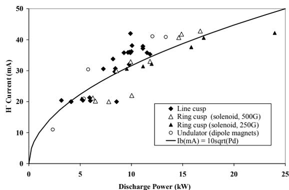
Figure 3. Measured  $H^-$  current as a function of the discharge power.  $R_{em} = 0.8\text{cm}$  in these measurements.
