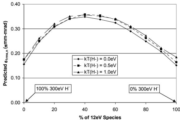
Fig. 7. PBGUNS model for emittance predictions of extraction of mixed-energy H<sup>-</sup> from a plasma source.
