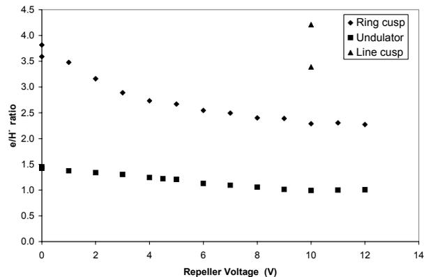
Fig. 2. The measured e/H<sup>-</sup> ratios for three different repeller magnet configurations.
