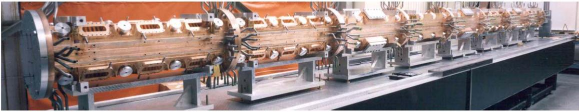
Figure 5: Eight-meter-long RFQ in the tuning laboratory. Adjustable slug tuners can be seen in this picture.
