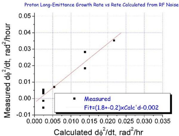
Figure 3: Plot comparing the measured longitudinal emittance growth rate to the emittance growth rate calculated based on the total spectral density of phase noise measured at the synchrotron frequency.
