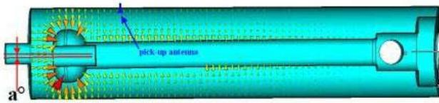
Figure 5: A cavity with bent central electrode.
