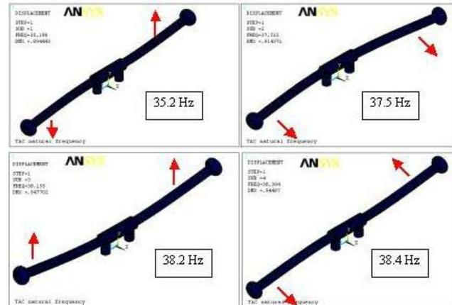
Figure 4: The modes of the central electrode mechanical vibrations.
