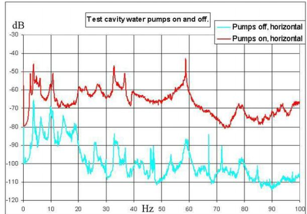
Figure 6: Comparison of mechanical vibration spectra with and without water pumps.
