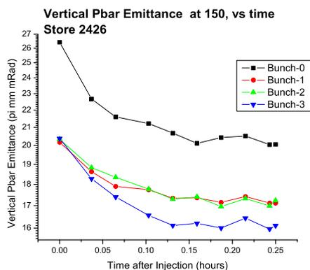
Figure 10: Drop in vertical emittance of the first four anti-proton bunches after injection in a recent store. The asymptotic emittance of each bunch is a measure of its dynamic aperture.
