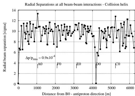
Figure 5: Beam separations at all the parasitics at 980 GeV with expected values for the proton momentum spread.
