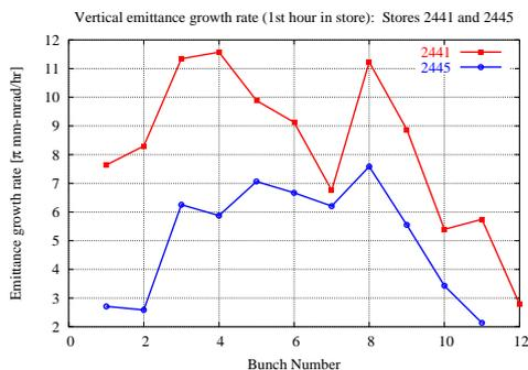
Figure 12: Bunch by bunch vertical emittance growth rates at the beginning of two recent stores. Lowering the vertical tune by 0.001 helped lower the growth rate in Store 2445.
