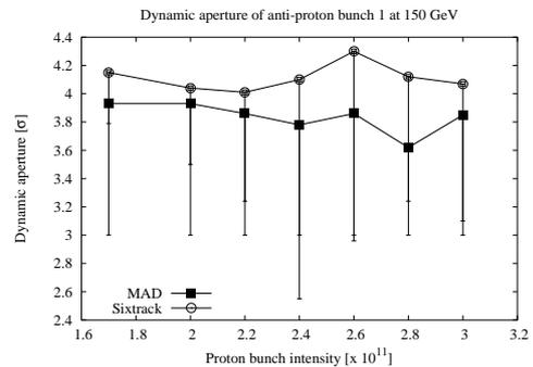
Figure 7: Dynamic aperture after  $10^6$  turns of anti-proton bunch 1 vs proton intensity at injection. The average value (over all angles in coordinate space) along with one-sided error bars to represent the minimum value at each intensity are shown.
