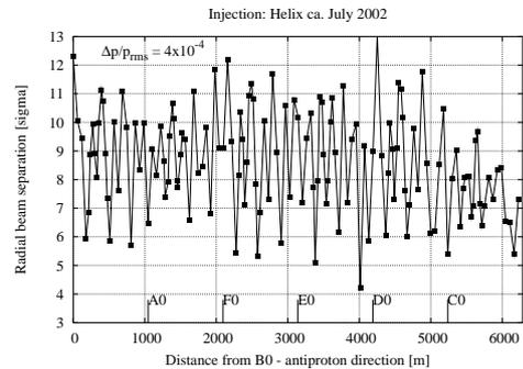
Figure 1: Beam separations at all the parasitics at 150 GeV with the design value for the proton momentum spread and the present injection helix.
