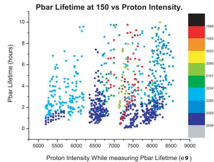
Figure 8: Lifetime of anti-proton bunches vs proton intensities in several recent stores.
