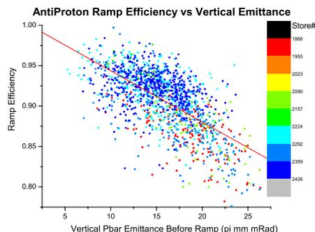
Figure 11: Anti-proton ramp efficiency vs anti-proton vertical emittance in several recent stores.
