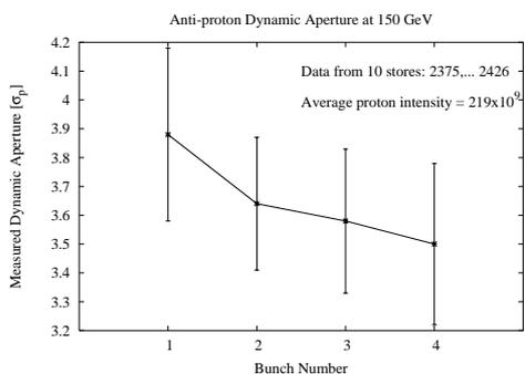
Figure 9: Dynamic aperture of the first four anti-proton bunches at injection calculated from the measured drop in emittance in 10 recent stores. The error bars represent the variation over the stores.
