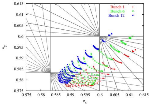
Figure 6: Tune footprints of bunches 1, 6 and 12 superposed on the 5th and 12th order sum resonances.
