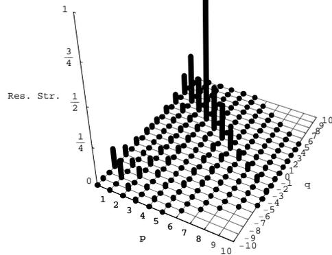
Figure 4: Resonance strengths at injection at an amplitude of  $2\sigma$  with lattice and beam-beam nonlinearities.
