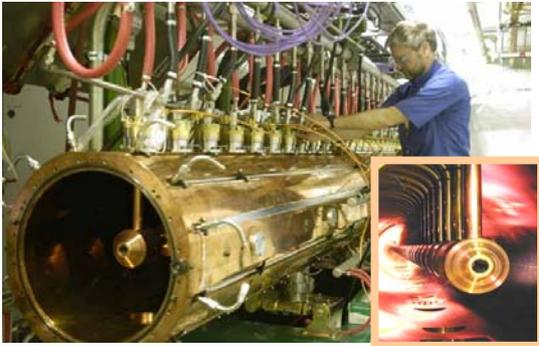
Figure 5: DTL tank 3 in the tunnel during final installation. Tank 3 contains 33 DTs.
