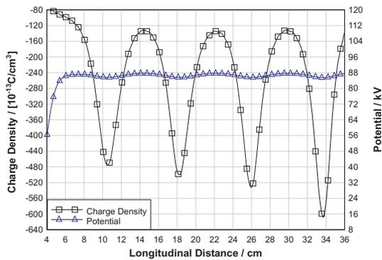
Figure 4: Charge density and potential on the gun axes.
