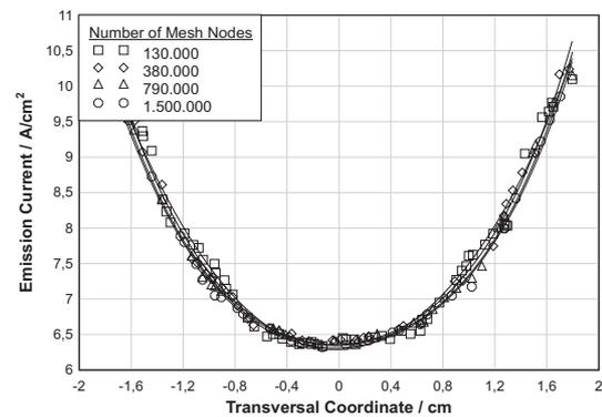
Figure 6: Emission currents on the source surface using the conformal method.
