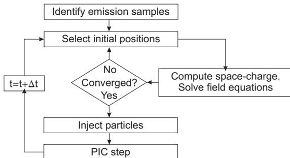
Figure 2: Simulation flow chart with particle injection.
