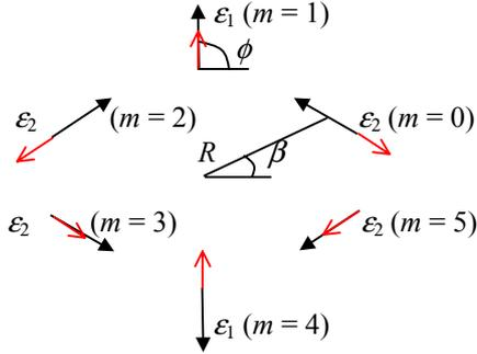
Figure 2: Skew quad nulling scheme, with field with design dipole orientation shown with red arrows and the nulling magnetization perturbations show in black.
