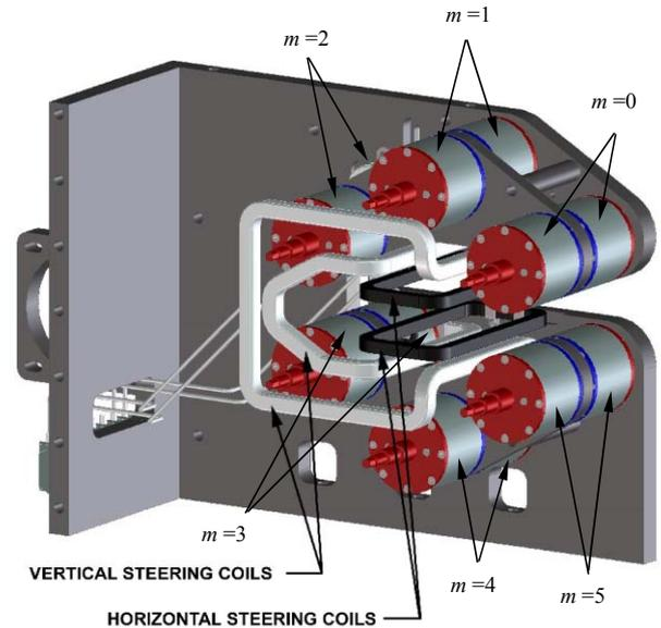
Figure 1: Chicane magnet tuners and steering coils
