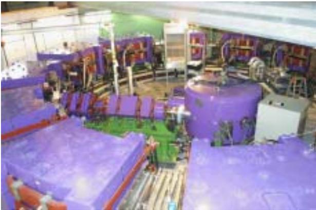
Figure 2: 150MeV FFAG ring and injection cyclotron
