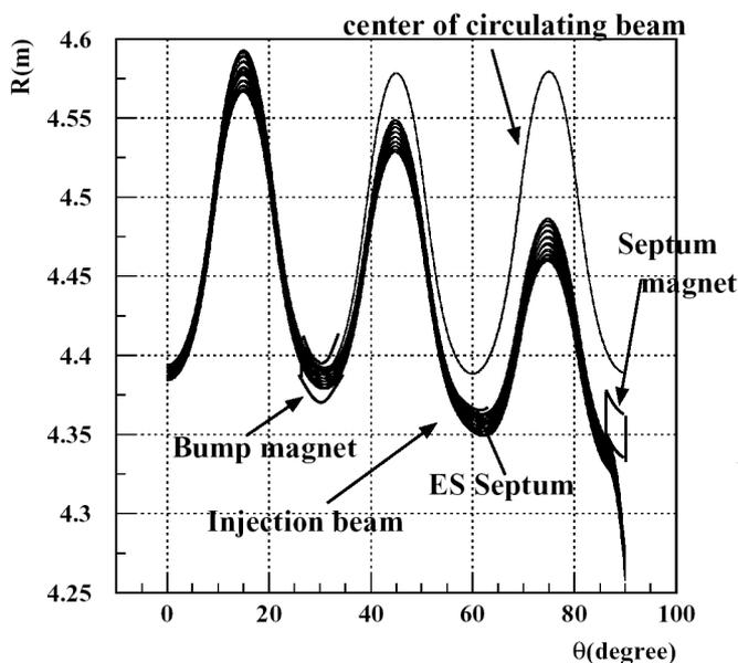
Figure 3: Injection Orbit of 150MeV FFAG
