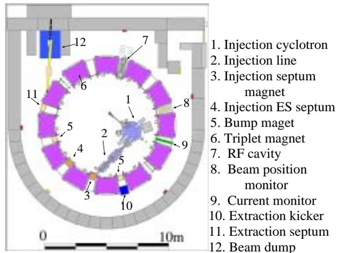
Figure 1: Schematic view of 150MeV FFAG
